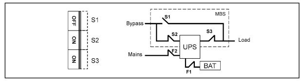
Figure 17 The normal (UPS supplying the load) positions of the three MBS switches.
